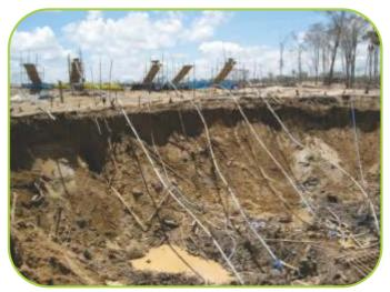
Figure 2. Extraction and washing of organic soil by alluvial gold mining
